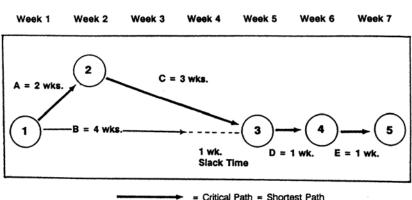
EJECTION SEAT SWITCH PROJECT CRITICAL PATH CHART
